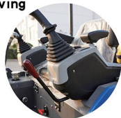
液压先导操作 Hydraulic pilot handle
