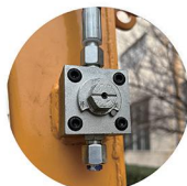
备用油管+截止阀 Spare Oil Pipe and Cut-off Valve
