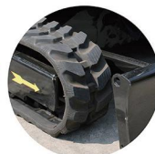
工程橡胶履带 Engineering rubber tracks
